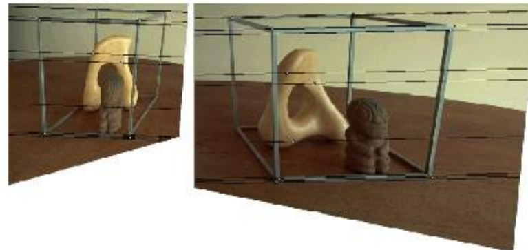
(b) Image pair transformed by the specialized projective mapping \mathbf{H}_p and \mathbf{H}'_p . Note that the epipolar lines are now parallel to each other in each image.
